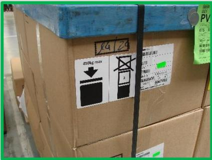
Designation of max. top load must be attached at one way packaging
